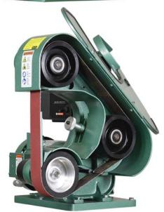
Adding only the 442-2 safety guard assembly does **not** provide sufficient protection from pinch points, and other rotational hazards. The owner of the equipment is urged to purchase the complete kit for compliance.
